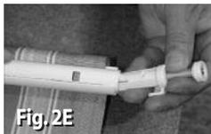
Insert the *Roller Sleeve* assemblies back into the *Bottom Cross Member*, ensuring that the locking tab engages the corresponding punched square hole in the *Bottom Cross Member* (Fig. 2E).
