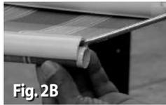
Remove the *Fabric Clamp*. To do this, insert a flat head screw driver between the canopy fabric and the *Fabric Clamp*. Pry upward to release the *Fabric Clamp* (Fig. 2B).
