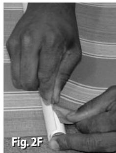
Measure the canopies to ensure the desired length is correct before trimming off excess canopy material. Remove the canopies and place on a flat, clean surface. To remove the excess canopy material, use the edge of the *Fabric Clamp* as a guide when cutting with a sharp utility knife (Fig. 2F).
