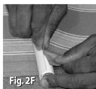
Insert the Roller Sleeve assemblies back into the Bottom Cross Member, ensuring that the locking tab engages the corresponding punched square hole in the Bottom Cross Member (Fig. 2E).
