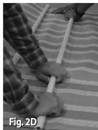
Place the Bottom Cross Member (aluminum) underneath the canopy, centering it on the two marks. Position the Bottom Cross Member so the punched square holes at the ends are facing downward. Holding the Bottom Cross Member in this position, reassemble the Fabric Clamp by snapping the Fabric Clamp in place at both ends and pressing down, working toward the center.
