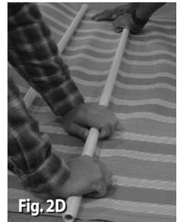
Place the *Bottom Cross Member* (aluminum) underneath the canopy, centering it on the two marks. Position the *Bottom Cross Member* so the punched square holes at the ends are facing downward. Holding the *Bottom Cross Member* in this position, reassemble the *Fabric Clamp* by snapping the *Fabric Clamp* in place at both ends and pressing down, working toward the center (Fig. 2D).
