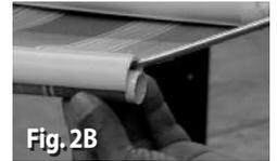
Remove the *Fabric Clamp*. To do this, insert a flat head screw driver between the canopy fabric and the *Fabric Clamp*. Pry upward to release the *Fabric Clamp* (Fig. 2B).
